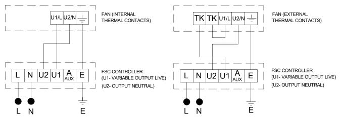
1-Fan terminals may vary with model. Refer to instructions supplied with fan for correct terminations.
