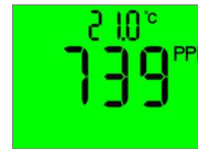
Diagram 4 When switch 2 is in the upward position with the Temp & RH Module attached then the RH will not be displayed.
