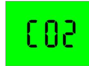
Diagram 2 When switch 2 is in the upward position the LCD will simply display 'CO2'.
