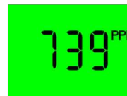
Diagram 1 When switch 2 is in the downward position then the CO2 level will be displayed.
