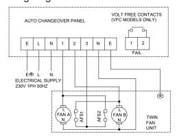
AFS1: Fan A airflow switch. Normally closed contacts that open when Fan A airflow is present
