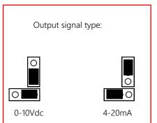
If the range links are incorrectly set, or missing the output range Will default to -10 to  $+40^{\circ}\text{C}$
